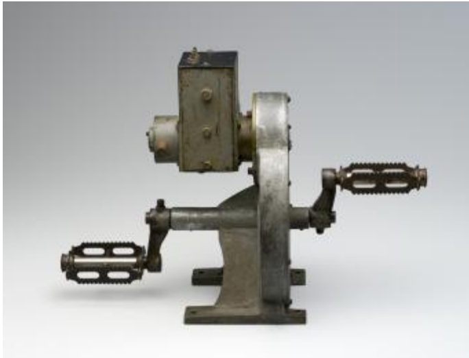
Figure 3: Alfred Traeger's Pedal Powered Radio (Powerhouse Museum)
