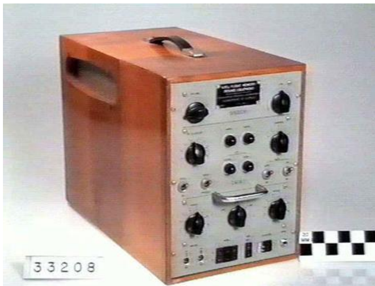
Figure 13: Prototype of black box flight recorder by David Warren (Museum Victoria)
